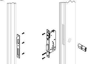
PASSO 3: FIXAR UMA DAS BASES DA ROSETA EM UM DOS LADOS DO PERFIL DO MONTANTE. DEPOIS DISSO, CLICAR A CAPA.
